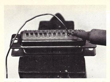
Photo 3. Tin each connector pin to be used. Solder should just fill the bottom of the solder pot.
